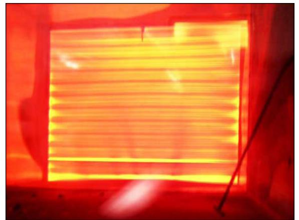
Damper blades glowing during a vertical fire test Fire dampers are exposed to temperatures approaching 1200 degrees celsius during fire testing, causing the galvanised steel blade pack to glow red hot.
