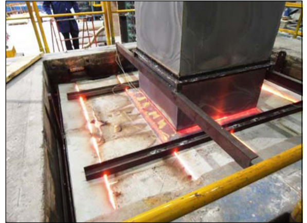
Series 100 fire damper during a horizontal fire test The test was stopped after 4 hours and 24 minutes because the 150mm thick concrete slabs themselves were failing. Damper leakage was actually decreasing at this stage.
