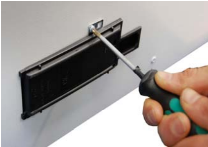
Remove the screw-earth of the connection box and disassemble from the equipment.
