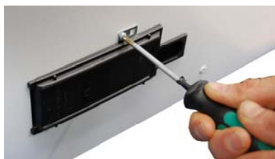
Remove the screw-earth of the connection box and disassemble from the equipment.
